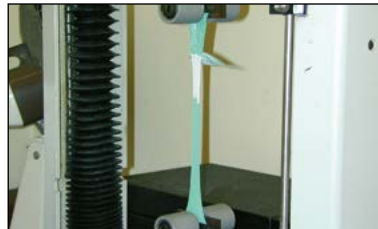
Peel bond strength (Delamination testing)
