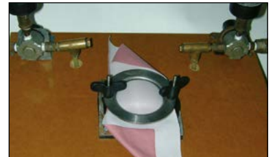
Static head pressure (Porosity testing)
